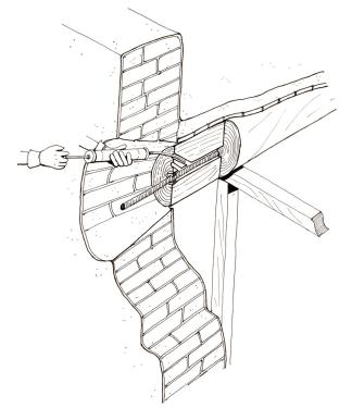
This drawing depicts the process of applying epoxy into the vent holes (step 20 of Method D).
